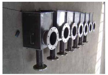
A deflector includes type II used for a cone roof tank and floating roof tank.
