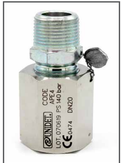
APE4: 3/4" NPT M SAFETY VALVE 140 bar OPEN-AIR DISCHARGE
